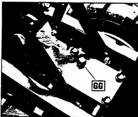
Fig. 2-11: Remove gear oil fill plug.
